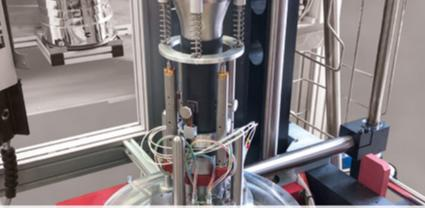
**COMPACT AND EASY-TO-USE INTERNAL INSTRUMENTATION** FOR DIRECT MEASUREMENT OF AXIAL AND RADIAL DEFORMATIONS OF SAMPLES: 4 AXIAL LVDTS + 4-BLADE CANTILEVER CIRCUMFERENTIAL EXTENSOMETER
